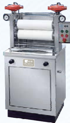
Model: P-B1 Padding Mangle Size: 125* 420mm Rollers: Horizontal Type
