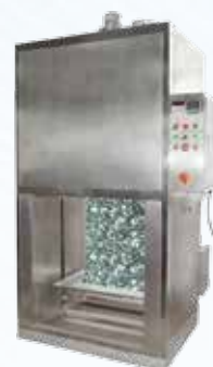
Sample Steamer Sample Size: 500*600mm*3pcs 1000*600mm*3pcs Temp.: Room Temp. ~ 180
