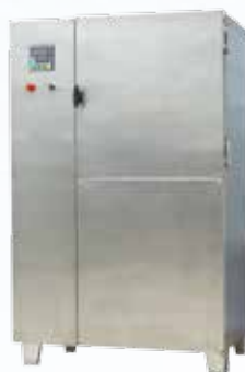
Steam Chamber Size: 480*400*480mm Temp.: 120°C Max
