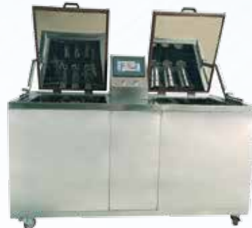
Colorfastness to Laundering tester with touchscreen Beakers: 10pcs*550ml + 8pcs*1200ml or 24pcs*550ml + 12pcs*1200ml [Relevant Standards] AATCC61/1A/2A/3A/4A/5A, JIS L0860/0844, BS1006,GB/T3921/1/2/3/4/5, ISO105C01/02/03/04/05/06/08, etc.
