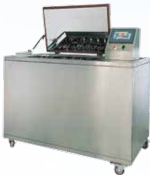
Colorfastness to Laundering tester with touchscreen Beakers: 10pcs*550ml + 8pcs*1200ml or 24pcs*550ml + 12pcs*1200ml [Relevant Standards] AATCC61/1A/2A/3A/4A/5A, JIS L0860/0844, BS1006,GB/T3921/1/2/3/4/5, ISO105C01/02/03/04/05/06/08, etc.
